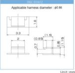
Example of wiring with clamp
